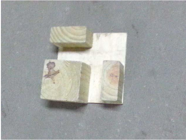
Figure E1. Landing framing jig.
