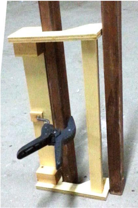
Figure E4. Baluster alignment tool Holds a baluster 4" from and parallel to the adjacent baluster.
