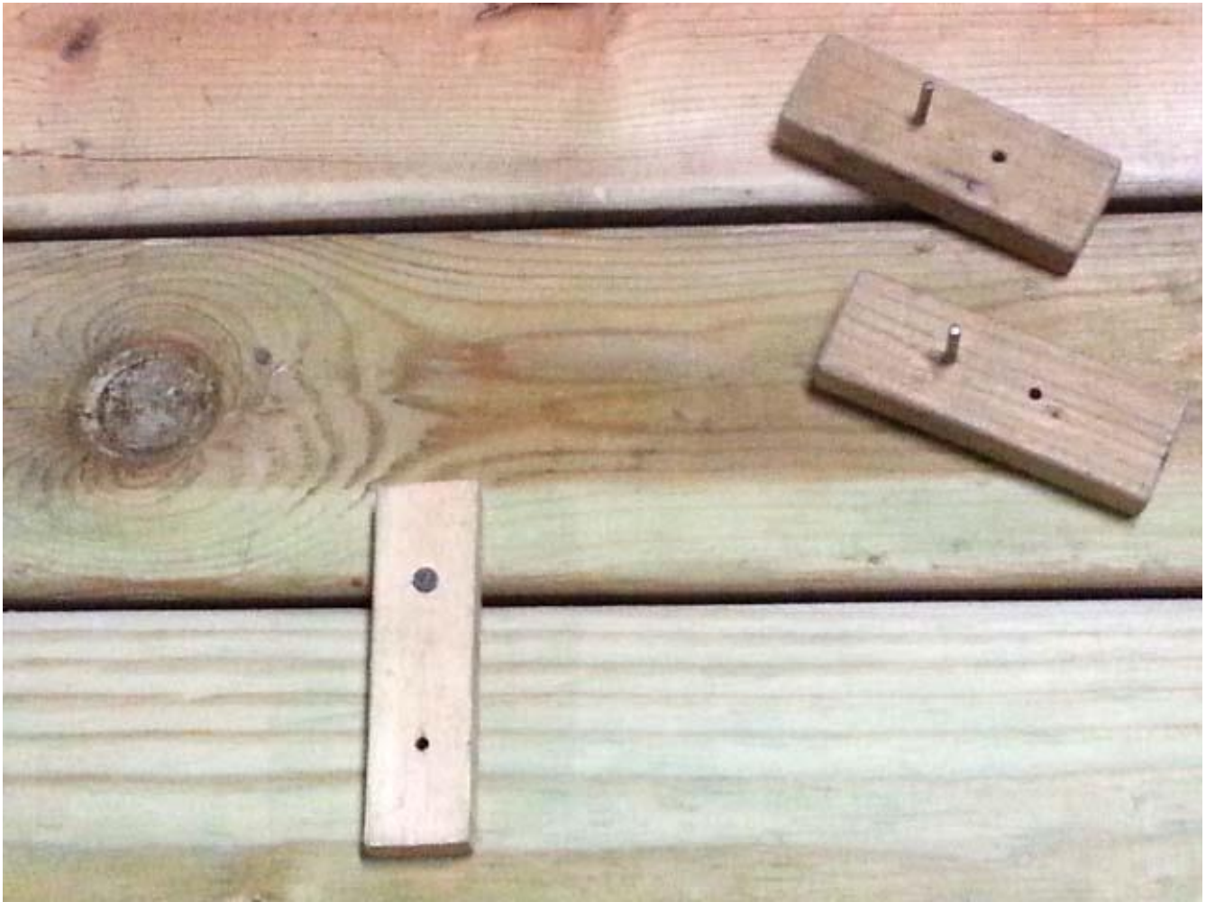
Figure E3. Deck board spacer. The spacer controls the deck board spacing while it is being screwed down. Two spacers are shown upside down.
